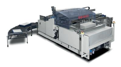
Automatic lining machine (cold vinylic glue and/or warm glue) High production equipment, no matrixes (clichés) need, no-stop paper loading from the top.
