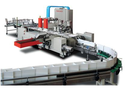
Fully automatic creasing (2 creases) and ring-metal riveting line. High production capacity equipment.
